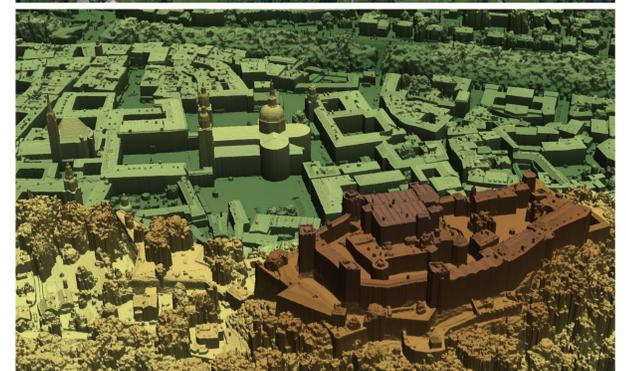
Textured 3D model: DSM is textured with nadir images for pixels on roofs, streets and ground while oblique images are used for facades.
