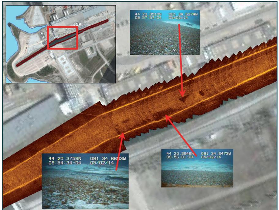
Horizontal forward-looking (eIQ mode) imaging surveys of the forebay bottom to identify accumulations of material (i.e. mussel shells) and to identify previous sediment removal sites. Inset photos show accumulation of mussel shells.
