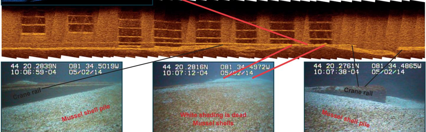
Vertical sonar imaging (Kongsberg M3 eIQ mode) of the intake wall (Unit 3). Also shown are the maintenance pump intakes at far left of sonar image. Note accumulation of material in front of the first four intake ports. Note the gap within the crane rail is partially hidden in accumulated material at the far right of sonar image.
