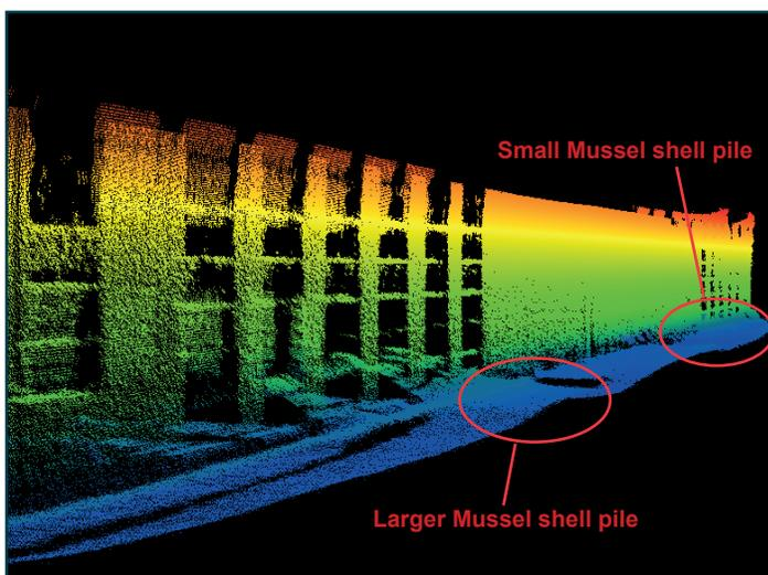
Detailed bathymetry (profiling and fast-profiling modes) of the intake channel, forebay bottom and forebay walls.
